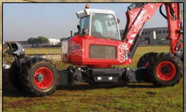
4 ruote sterzanti indipendenti 4 steering and independing wheels 4 roues directrices ind pendents
